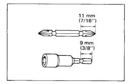
To install the bit, pull the sleeve in the direction of the arrow and insert the bit into the sleeve as far as it will go. Then release the sleeve to secure the bit.
